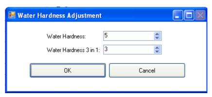
You can then change the value of "Water Hardness" and "Water Hardness 3 in 1" parameters. The typical range of possible values is between 1 and 10. The maximum possible value depends however on the actual configuration of the dishwasher.
