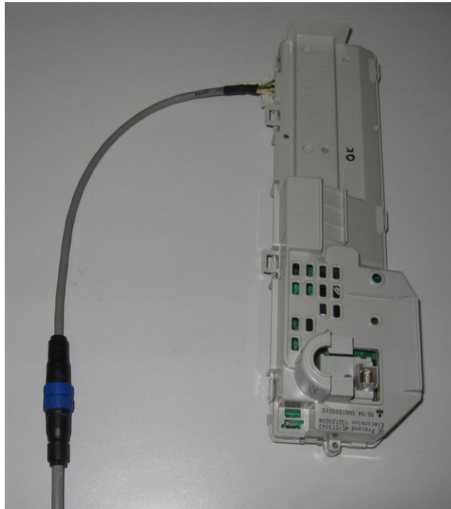
Fig. 21. Board with appliance cable connected
