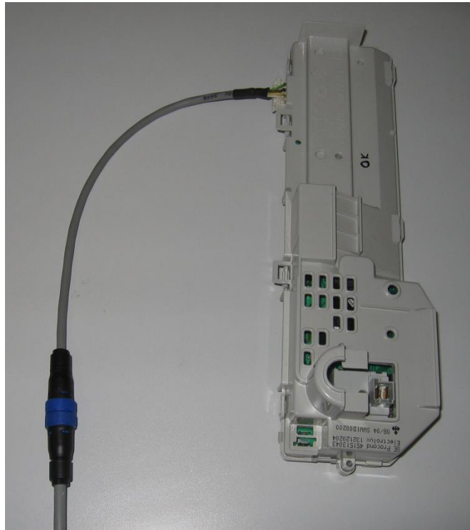
Fig. 20. Board with appliance cable connected
