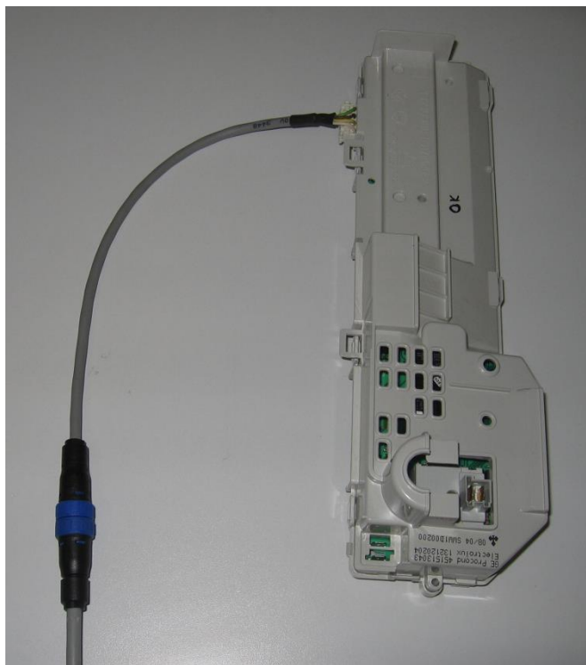
Fig. 20. Board with appliance cable connected
